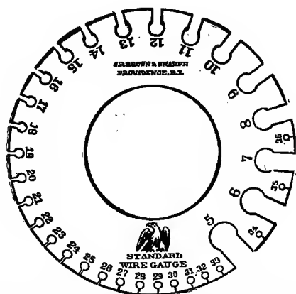
FIG. 259a.—Circular gauge, showing approximate dimensions of the wire measures on the American, or Brown & Sharpe, Wire Gauge System.
